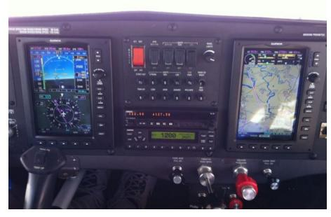
To the left you see our 'in flight' view. The left display looks like an F15 with synthetic vision. The right screen shows engine detail and a moving map. Between them is circuitry, comm-radio and Mode C. No round dials.
