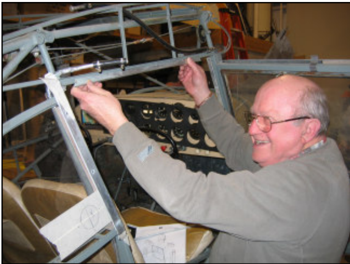
Curt Lockrem is trial-fitting parts of the forward door frame.
