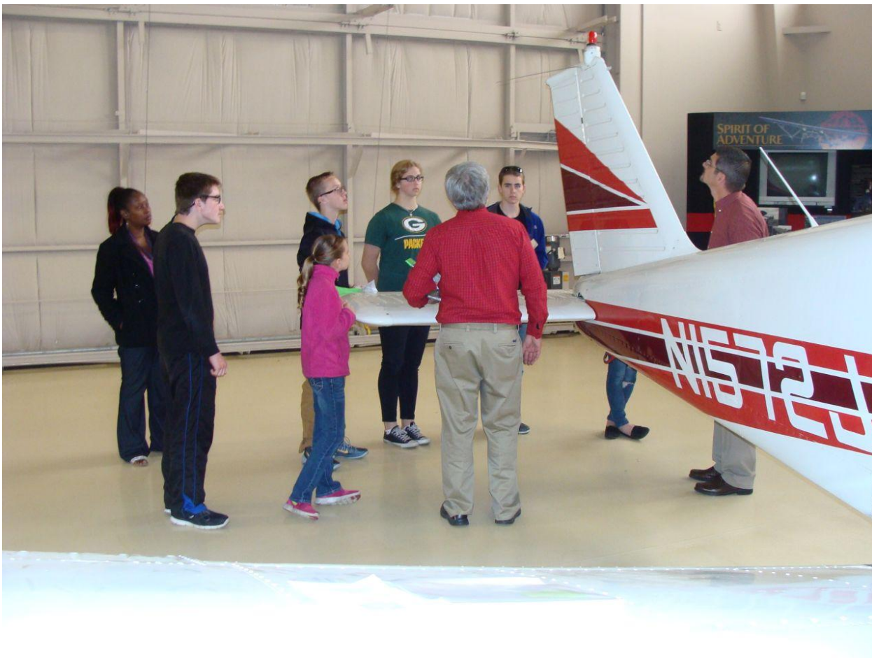
EAA 838's Carl Bumpurs explains how the empennage controls two of the three axes of an airplane. ('Empennage' is French for 'feathers on an arrow')
